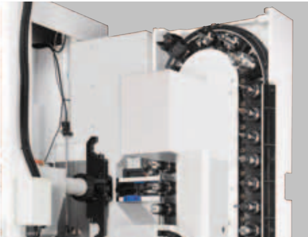
Capacity of standard tool magazine may contain up to 36 cutters while the optional one has 72 cutters. The TM-2500 series may select tool specifications according to customer requirements.
